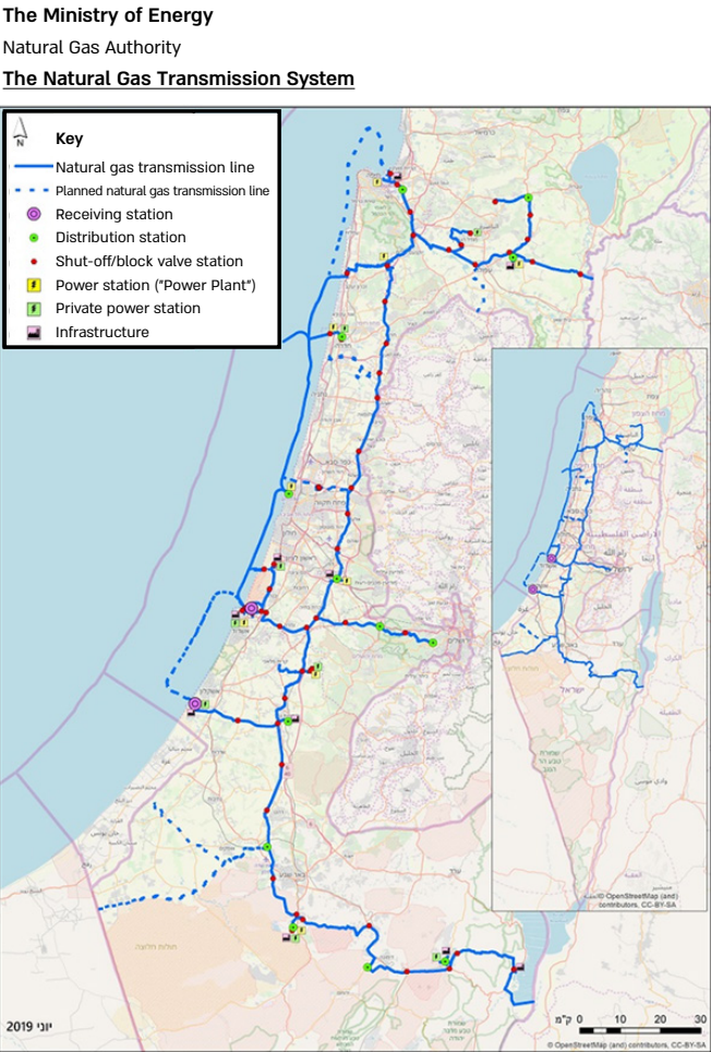
FIGURE 5. THE NATURAL GAS TRANSMISSION SYSTEM
