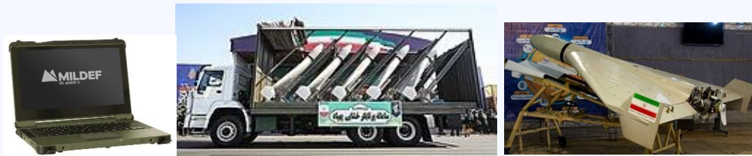
Figure 3. Components of a Typical Loitering Munition Weapon System
