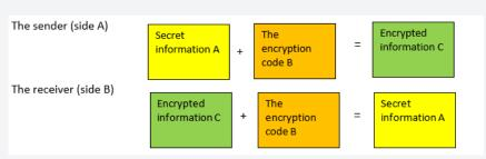
Illustration 1: Schematic Description of the Encryption Principle
